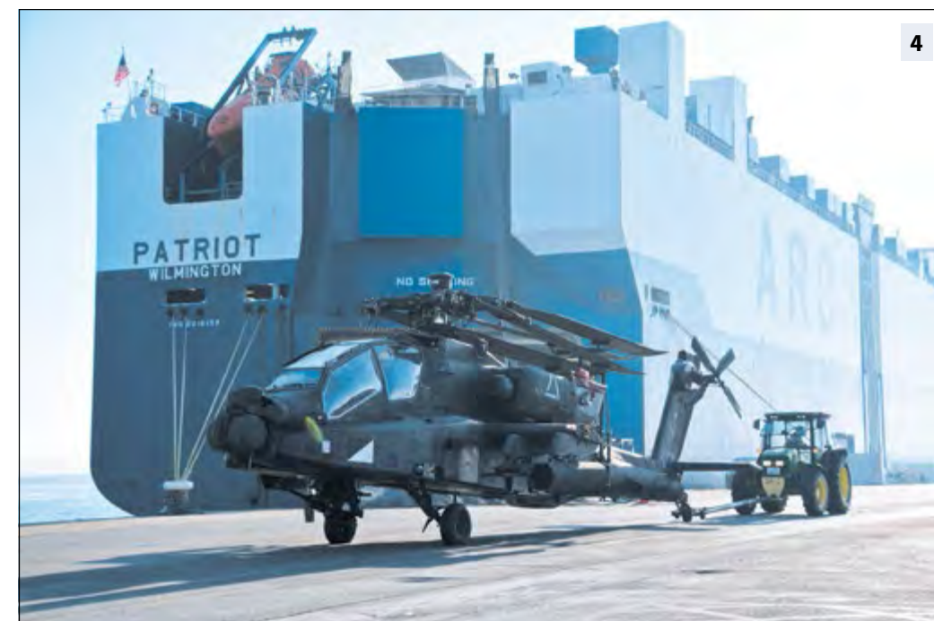
4) An AH-64D Apache helicopter is taken off a ship at Naval Station Rota, Spain, during helicopter intermodal operations. This operation uses multiple modes of transportation to reduce cargo handling, improve security, minimize damage and allow quicker freight transportation.
